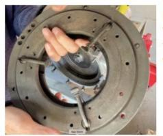
with 'mousetrap' springs and spigots was very difficult, until I realised I could fit the 'mousetrap' spring on the toggle arms
