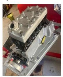
Next came the fitting of the Cylinder Head. I had bought an 'Alta' aluminium cylinder head
