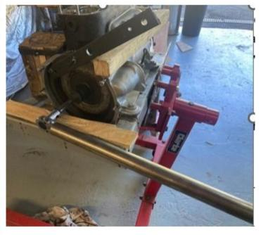
earlier in the year, and now I realised I need to check that there was sufficient clearance for the valves when they were fully open. I did a quick check without the gasket in place – all was well-so
