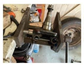
Using a vice and sockets to push the old bushes out, I also used a bolt and nut to pull them out.
