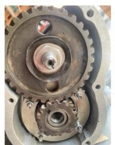
Note the '0' s – two on the cam pinion and one on the crank pinion which need to align as shown.
