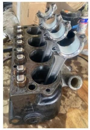
A trip to the Le Mans Classic in my MGA interrupted progress for a while, but I soon had the front cam and crank pinions on, and tightened up. The crank being locked in position with a steel plate and a long length of steel whilst I leaned on the dog nut with a big socket in my
